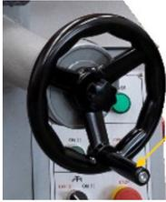
A close-up photograph of a black hand wheel handle being attached to a metal shaft. A yellow arrow points to the handle, labeled with the number '1'.                                                  | <b>Assemble hand wheel handle</b> <ul style="list-style-type: none"><li>• Screw the handwheel handle into the thread of the hand wheel height adjustment Z-axis</li></ul>                                                                           |
